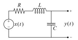
This is an example of an *RLC circuit*, and in this project we will investigate the role such a circuit can play in signal processing. We will consider the (time dependent) voltage source x(t) as the input signal to the circuit, and the voltage y(t) across the capacitor as the output.
